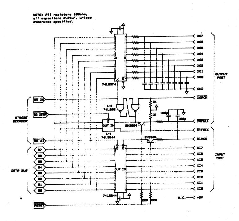
Fig. 5-2 Modified Minimal Interface
